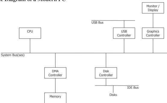
Master / Slave control system – CPU is the master controller. DMA, Disk, USB, Graphics controllers are the slave controllers and interrupt the CPU, through the OS, that it is done performing an action.
